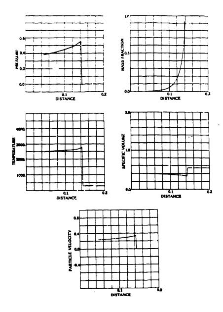
Fig. 1. The high resolution one-dimensional reaction zone profile of PBX-9404 calculated using the SIN code.
