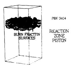
Fig. 5. Burn fraction surface profiles after reaction zone interacts with heterogenities in PBX-9404.
